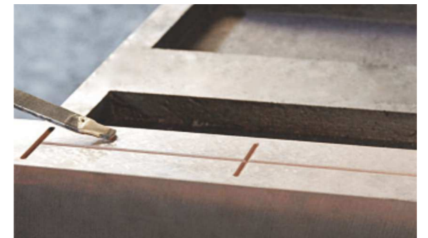
机床导轨运动面进行精密铲配 Machine Tool's Motion Surface Experiences Precise Scraping
